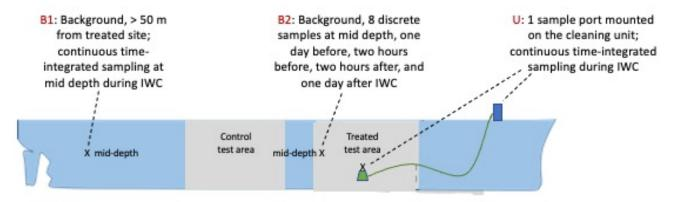
Figure 6. Diagrammatic example (not to scale) of the locations of the three water quality sampling sites: U, B1, and B2. This sampling scheme represents 10-11 samples total, with each analysis conducted in triplicate to quantify analytical variance.
