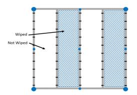
Figure 3. Quadrats are used to determine biofilm cover by using percent cover visual estimates and fouling ratings within the four bands. The two quadrats bands identified in blue will be spongewiped of biofilm. Side-by-side photos will compare wiped versus not wiped sections.
