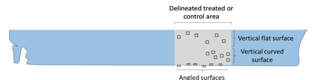
Figure 2. Pictorial representation (not to scale) of a delineated treated or control area (grey), surface types within the cleaning area (named), and six replicate plots within each surface stratum (black boxes). The bottom area, not visible in this figure, will also be sampled in six replicate plots.
