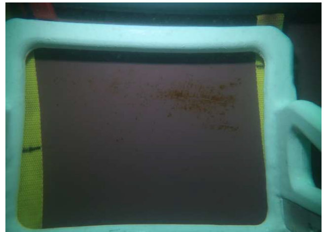
Figure 4. Pictures from the second photo survey in March 2022. A) flat untreated, B) flat treated, C) Curved untreated, and D) curved treated. The brown coloration is biofilm present on the hull, FR 20 or less.
