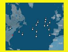
Fig. 1 Location of ballast-tank ocean exchange for the 14 of 17 ships reporting exchange. The port of Norfolk, Virginia (USA) is indicated by a red dot.
